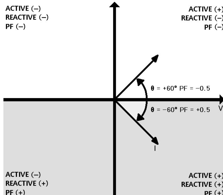
\*the reactive power measurement is negative when the load is capacitive, and when the load is inductive. The sign of the reactive power can therefore be used to reflect the sign of the power factor.
